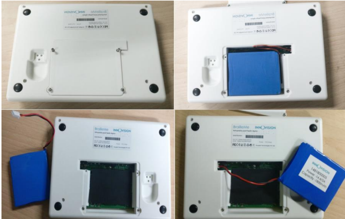
Images of the 4 steps of battery replacement
