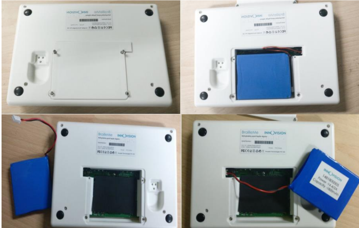
Images of the 4 steps of battery replacement
