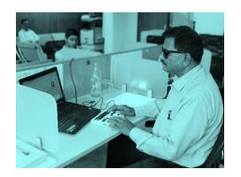
BrailleMe has a fast, smooth 20 cell 6-dot Braille display designed to give paper like crispness. It has a Brailler style keypad and cursor buttons for dynamic typing. It is ideal for students for easy access to books and note-taking. It is also well suited for working professionals with compatibility with computers & screen readers for a combination of Braille and audio for a seamless experience.
